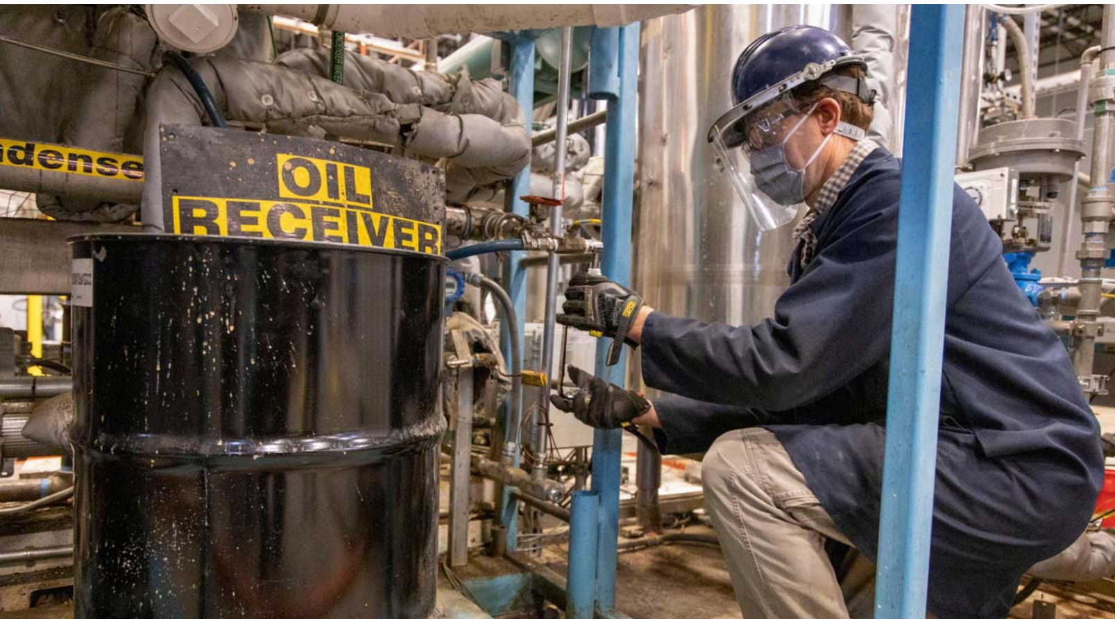
FBRI researchers use mixed acids derived from sawdust to produce thermal deoxygenation (TDO) oil in the Synthetic Crude Oil Pilot Plant.
