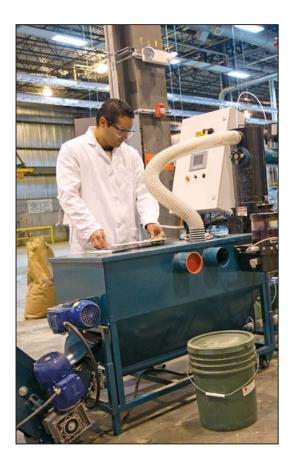
t current energy costs, pellet stoves have become a popular method for heating homes and small business, providing a clean method of heating with renewable energy sources. Almost any plant material can be made into pellets and new raw material sources are frequently advocated. Proof of suitability of new sources can be easily accomplished with the Lawson Mills Pellet Mill.
