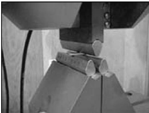
Fig. 5. Close-up of ILSS test of a FRP composite short-beam specimen.
