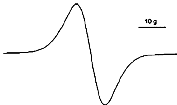
Fig. 2. Typical ESR spectra of phenoxy radicals on solid state fibers.
