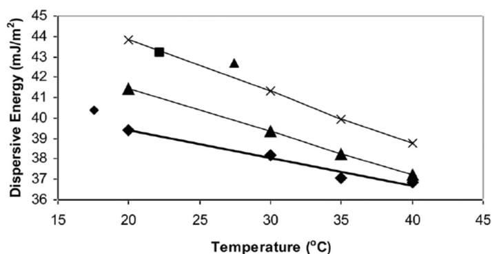
Figure 6. Dispersive surface energy calculated by the Schultz method for extracted maple residues, ♦ is control, ▲ is SF-3.54, and × is SF-3.81.
