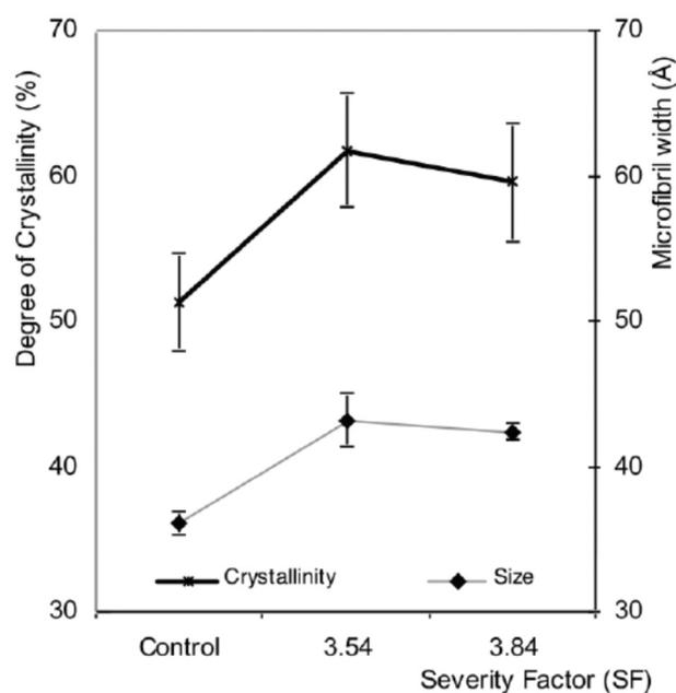
Figure 5: Crystallinity degree - microfibril width behavior of red maple control and two severity factor in hot water treatment at 160°C.
