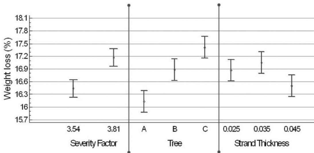
Figure 1: Effect of severity factor (SF), tree source, and strand thickness on weight loss during hot water extraction at 160°C (Paredes et al., 2008a).
