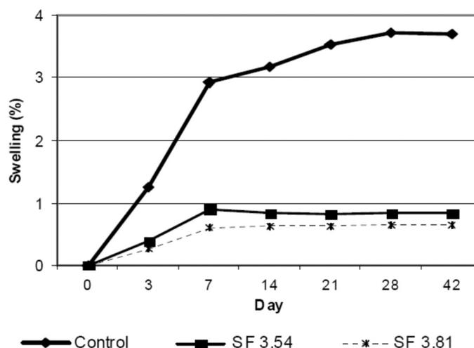
Figure 2: Panel thickness increase occurring from out of press to equilibrium conditions (23 C/ 65% RH).
