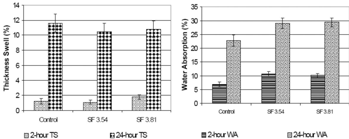
Figure 3. Thickness swell and water adsorption response of red maple control and hot water extracted panels OSB (Paredes et al., 2008a).
