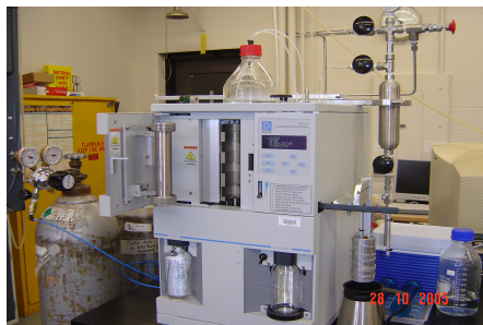
Figure 1. Modified Accelerated Solvent Extractor (ASE-100)
